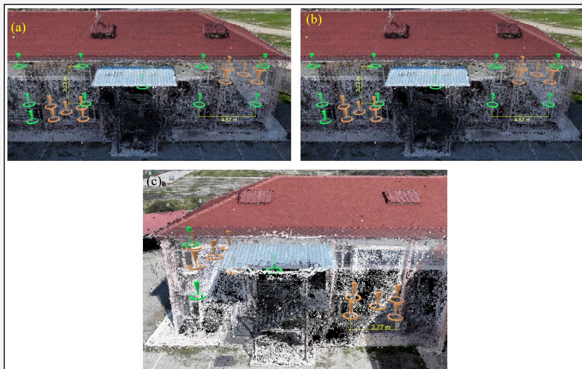
Figure 5. Enhanced point cloud view data of surfaces 1, 2, and 3 generated from the hybrid photogrammetric model: (a) Surface 1 heading east, (b) surface 2 heading north, and (c) surface 3 heading west are represented respectively. The green markers indicate the detail points used in the point- and length-based comparisons, whereas the brown markers indicate the representative points selected for the surface-based comparison. Approximate local scale indicators were added using known façade distances between clearly identifiable reference points on the same wall plane
