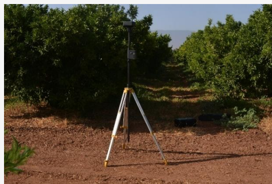
Figure 3: DJI D-RTK 2 base station used to support RTK-based direct georeferencing during UAV image acquisition
