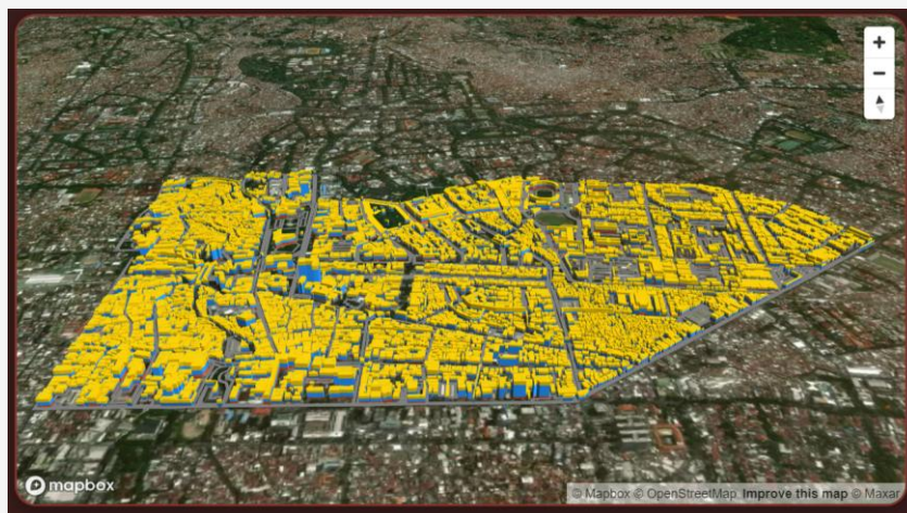
Figure 5: Overlay of the generated voxel model on top of the original 2D cadastral map of Sumur Bandung District rendered on a Mapbox satellite base layer
