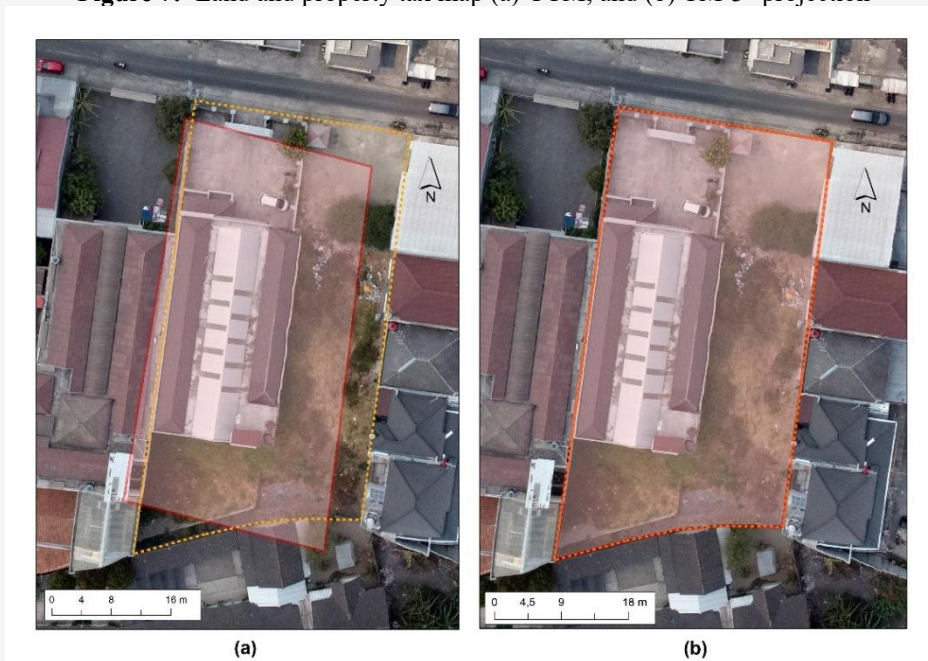
Figure 8: (a) Land parcels of the LPTM before and (b) changes were made using the Replace Geometry Tool
