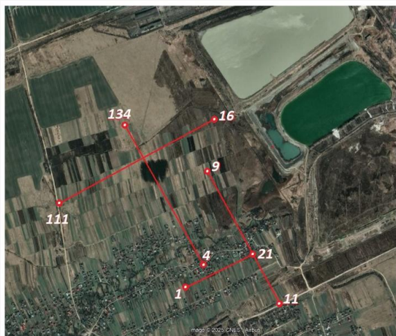
Figure 6: The levelling scheme over the Novo-Holyn mining field and the number of end-line benchmarks
