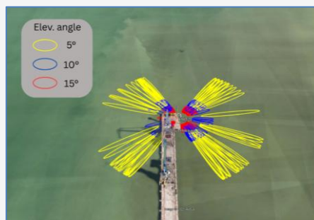
Figure 2: Reflection zone at station plotted by azimuth angle assuming reflector height is 5 meters
