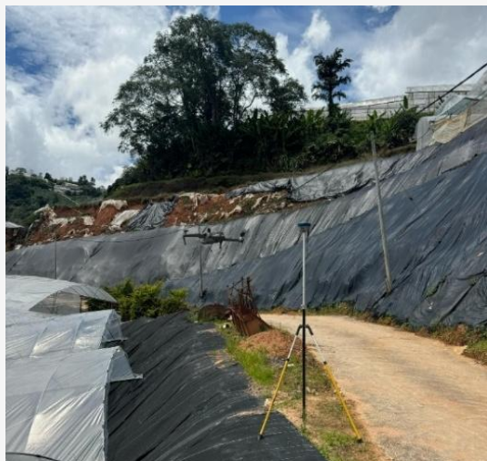
Figure 3: Data observation of a GCP and UAV drone
