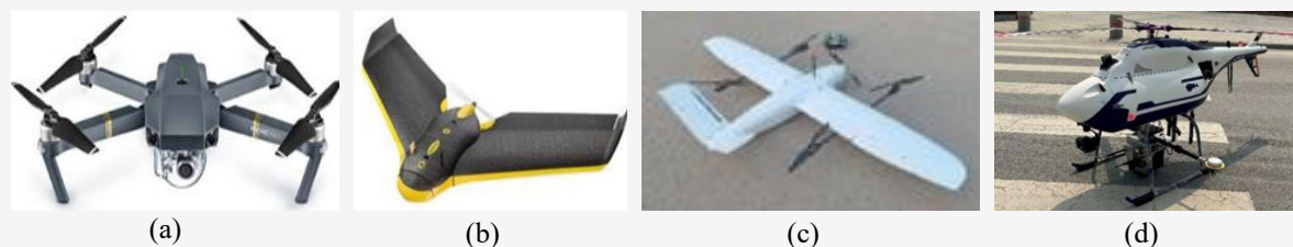
Figure 6: UAV platforms: (a) Multi-rotor UAV [2] (b) Fixed-wing UAV [52] (c) Hybrid UAV [75] and (d) Unmanned Helicopter [74]
