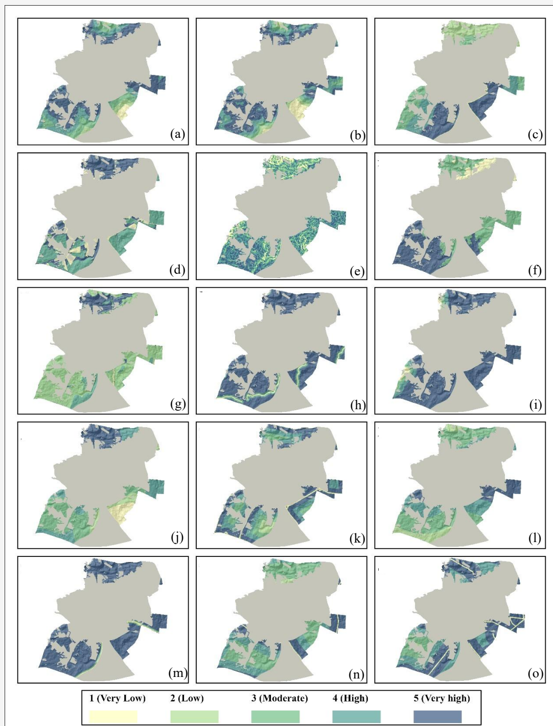
Figure 3: Maps of criteria: (a) proximity to amenities and facilities, (b) proximity to existing residential areas, (c) proximity to industrial areas, (d) land Use, (e) slope, (f) elevation, (g) geological characteristics, (h) proximity to hydrographic network, (i) proximity to forests, (j) AOD, (k) proximity to major roads, (l) proximity to tramway, (m) proximity to railway, (n) proximity to gas pipeline, and (o) proximity to the electrical grid
