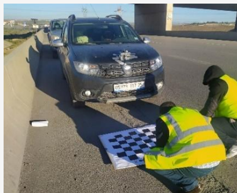
Figure 11: Smartphone camera calibration with Checkerboard Pattern
