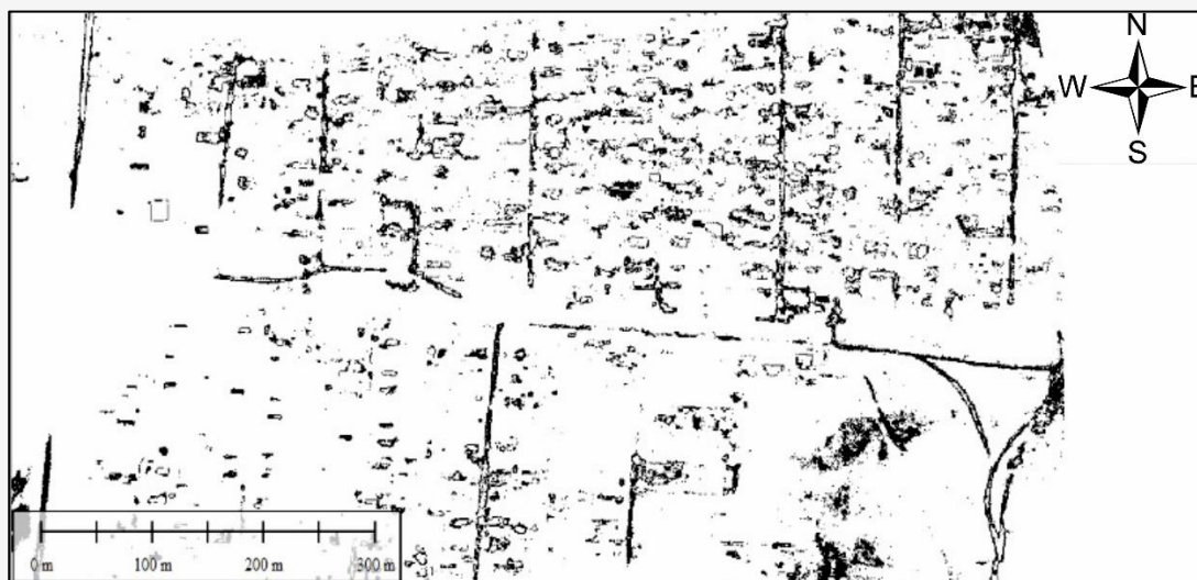
Figure 11: Unsatisfactory difference indicators of destruction were obtained after applying two groups of filters of space images
