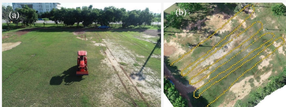
Figure 8: Visualization of tractor movement patterns, (a) the tractor testing in the field, (b) high-precision tracking results from the Low-Cost GPS and IoT system in agricultural field operations
