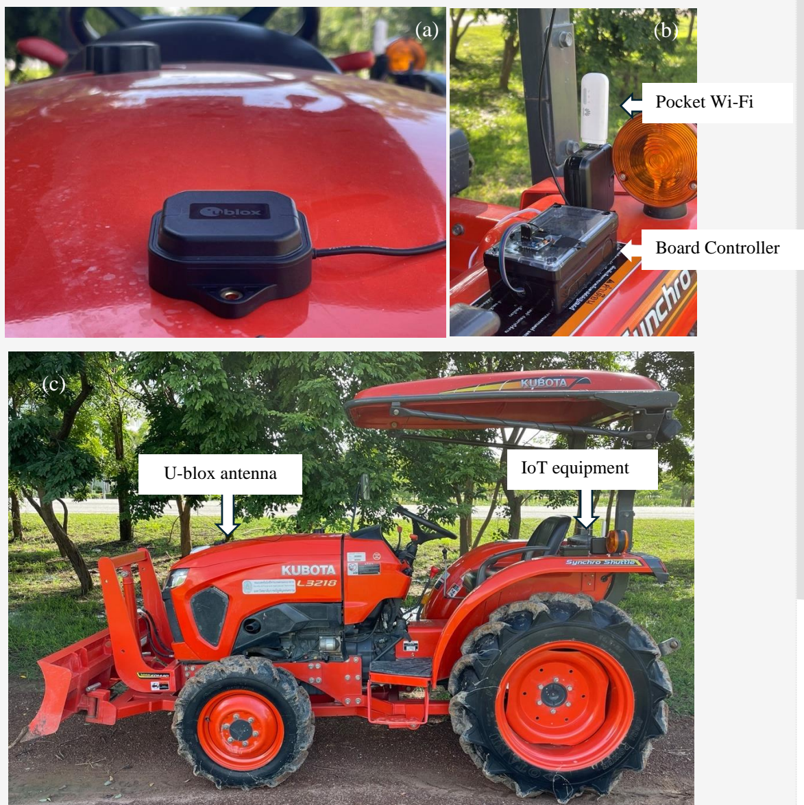
Figure 7: Components of the Low-Cost GPS and IoT system for agricultural tractor positioning: (a) U-blox NEO-M8N GPS module with antenna, (b) integrated IoT equipment set for GPS signal reception and data transmission and (c) equipment installation location on the tractor
