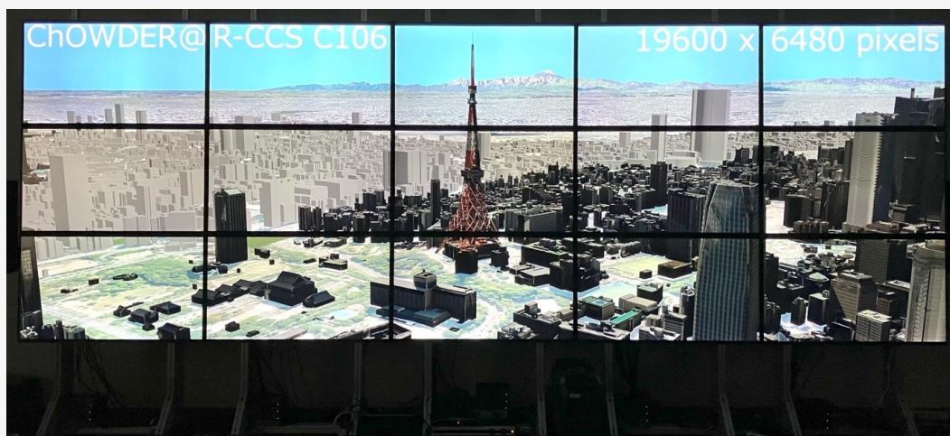
Figure 1: An example of viewing 3D geographic information by ChOWDER's 3DWebGIS distributed rendering method on a 20K horizontal resolution tiled display wall consisting of fifteen 43-inch 4K liquid crystal displays and fifteen PCs
