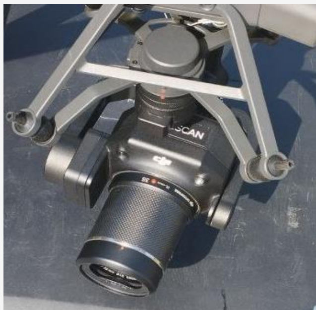
Figure 4: DJI Zenmuse P1 digital aerial camera mounted on the UAV gimbal
