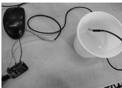
Figure 9: Implementation of DS18B20 is done with the help of NodeMCU
