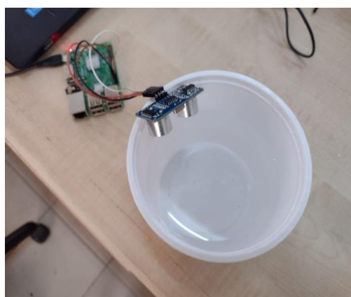
Figure 17: Ultrasonic sensor with Raspberry Pi
