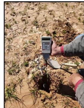
Figure 2: Soil Moisture Content (SMC) in-situ measurements. The left panel shows a photo of the Wadi where the 20 measuring locations exist and the right panel was taken during a measurement
